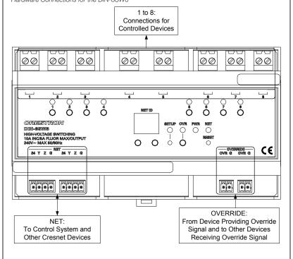
With the circuit breaker turned off, connect the wires to the terminal blocks per the markings provided on the DIN-8SW8.
